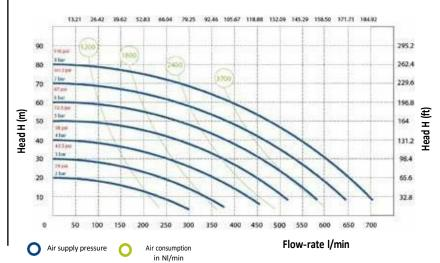
The curves and performance values refer to pumps with submerged suction and a free delivery outlet with water at  $20^{\circ}\text{C}$ , and vary according to the construction material.
