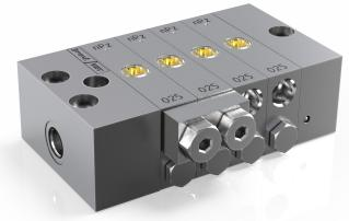
DropsaVET NPZ is a distributor that utilises the progressive movement of pistons to dispense precise amounts of lubricant to multiple lubrication points.
