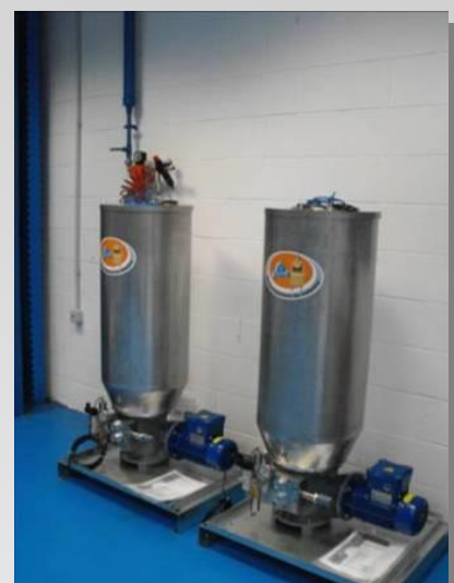
SUMO ATEX Stainless 316 version with Ex d motor Reservoir.
