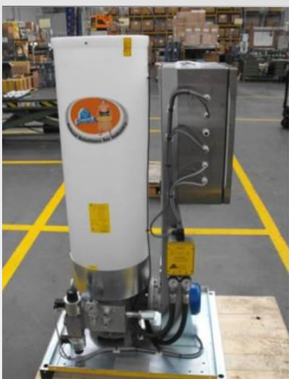
SUMO Pump semi-transparent reservoir with end of line pressure switches and control panel in a stainless box installed on the standard pallet
