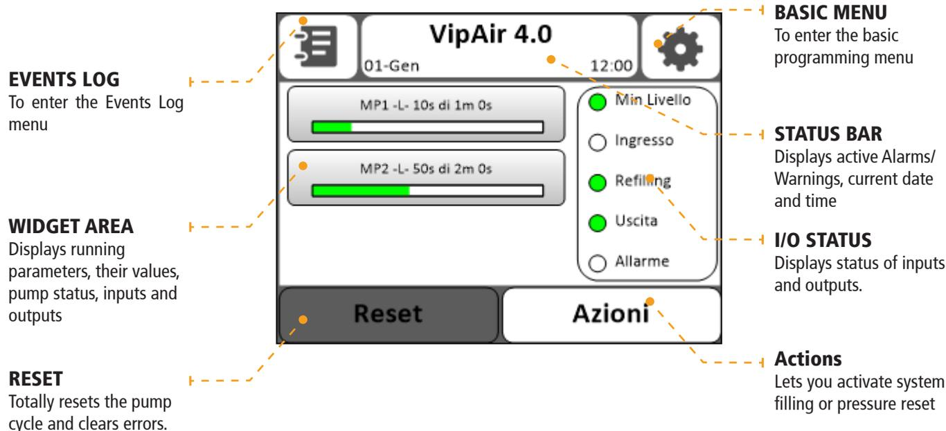
Press the middle of the screen (Widget Area) to view other system statuses; instead, press the top part of the screen (Status Bar) to display additional information regarding the status of the alarm/warning present.
